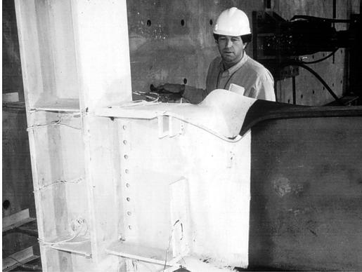
***Engineers expect steel to be ductile, capable of extensive bending and deformation without fracturing, as shown in this test specimen. The development of cracks in the steel at relatively low levels of loading was unexpected.***
