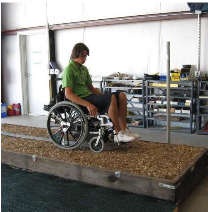
The "wheelchair test" is conducted on a sample test bed in the lab to determine the results for ASTM F1951-99.
