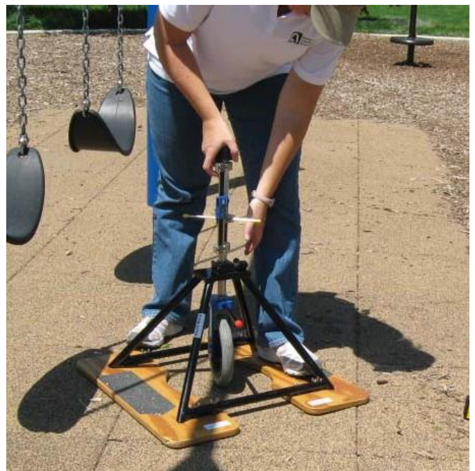
A Rotational Penetrometer (RP) is used here to measure the firmness and stability of the surfaces.
