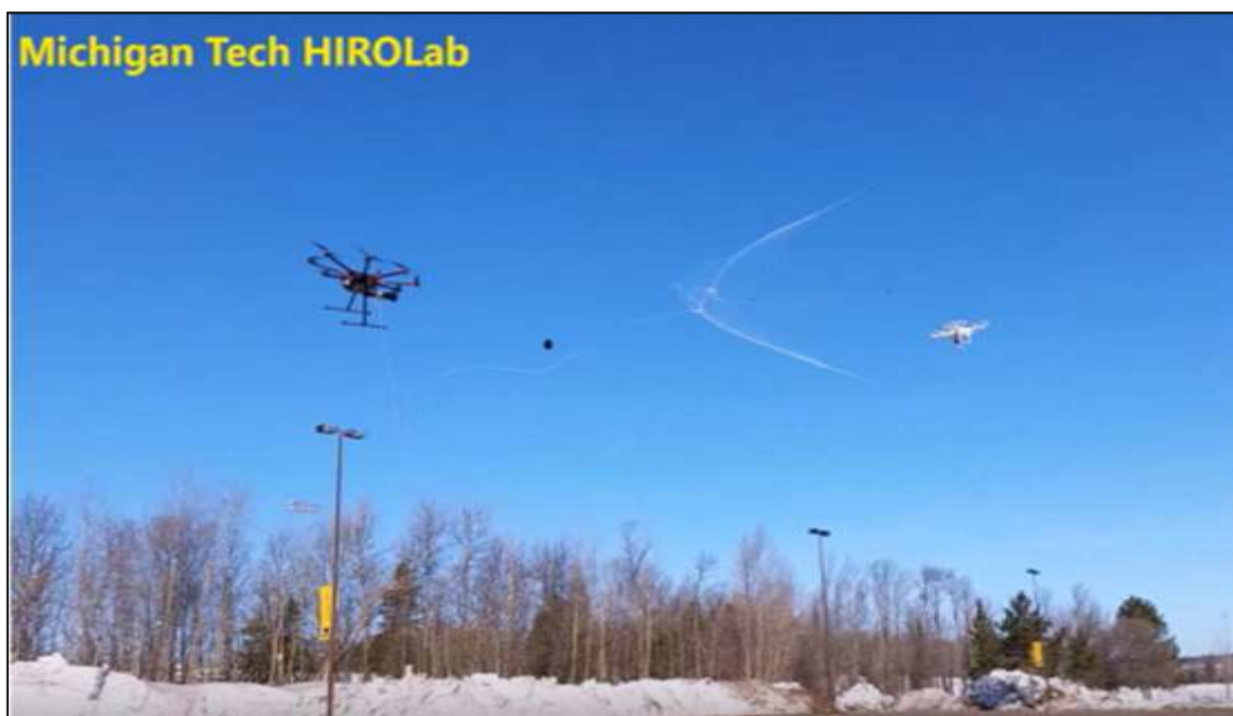
Figure 18. Robotic Falconry Prototype Drone-Catcher System 42
