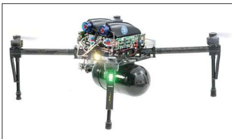
Figure 3. Intelligent Energy’s Ultra Lightweight Fuel Cell System 10
