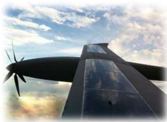
Figure 8. Solar-powered Silent Falcon sUAS 18
