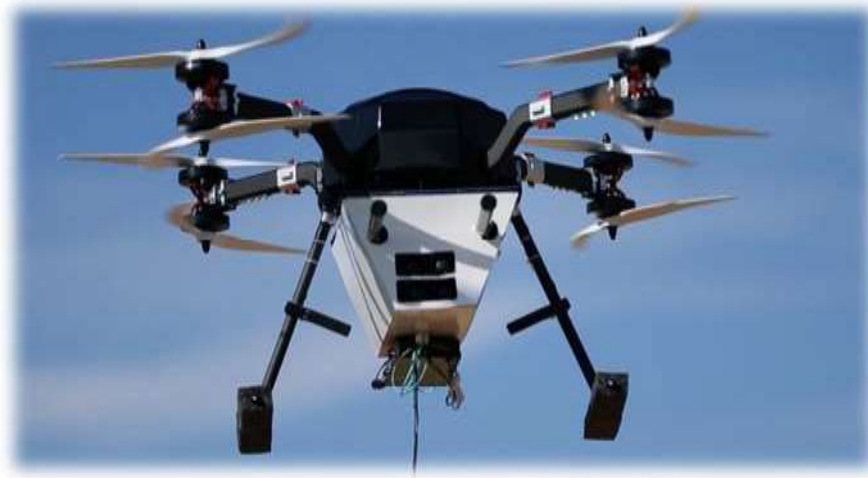
Figure 9. AT&T Flying Cell on Wings (Flying COW) 20
