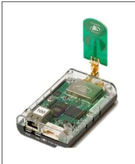
Figure 16. PulsON® 440 smart sensor 38
