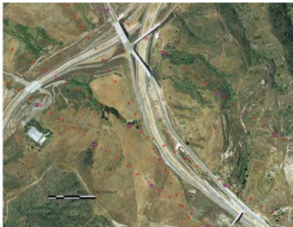
Figure 16. Photo. One-second GPS solutions are interpolated to obtain positions at the camera exposure centers.
