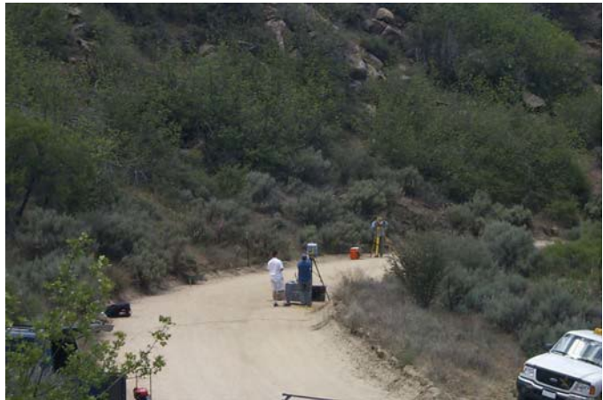
Figure 9. Photo. The brushy hillside directly facing the scanner provided limited success seeing to the ground surface.
