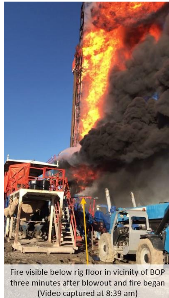
Figure 51. Video still of Patterson Rig 219 fire, taken 3 minutes after blowout began.
