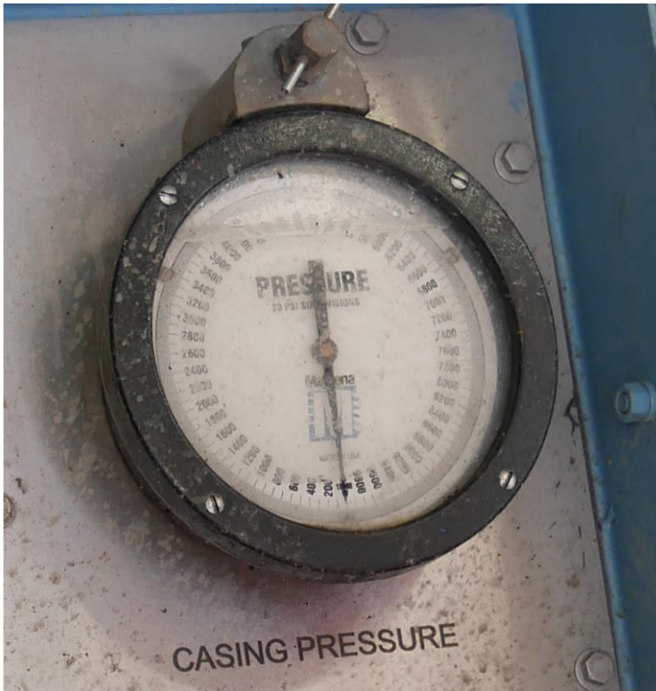
Figure 16. Photo of casing pressure gauge on an exemplar Patterson drilling rig. The pressure gauge could indicate pressures up to 10,000 psi. Low pressures might have been difficult to read on the Rig 219 pressure gauge, or the pressure gauge might not have worked properly at low pressures. The valve on the choke system (“HCR valve”) that needed to be opened to measure annular pressure might have been closed during pressure readings, or the line might have been plugged.
