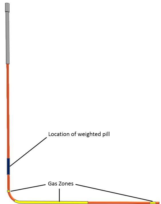
Figure 21. Depiction of well with gas zones and location of weighted pill.
