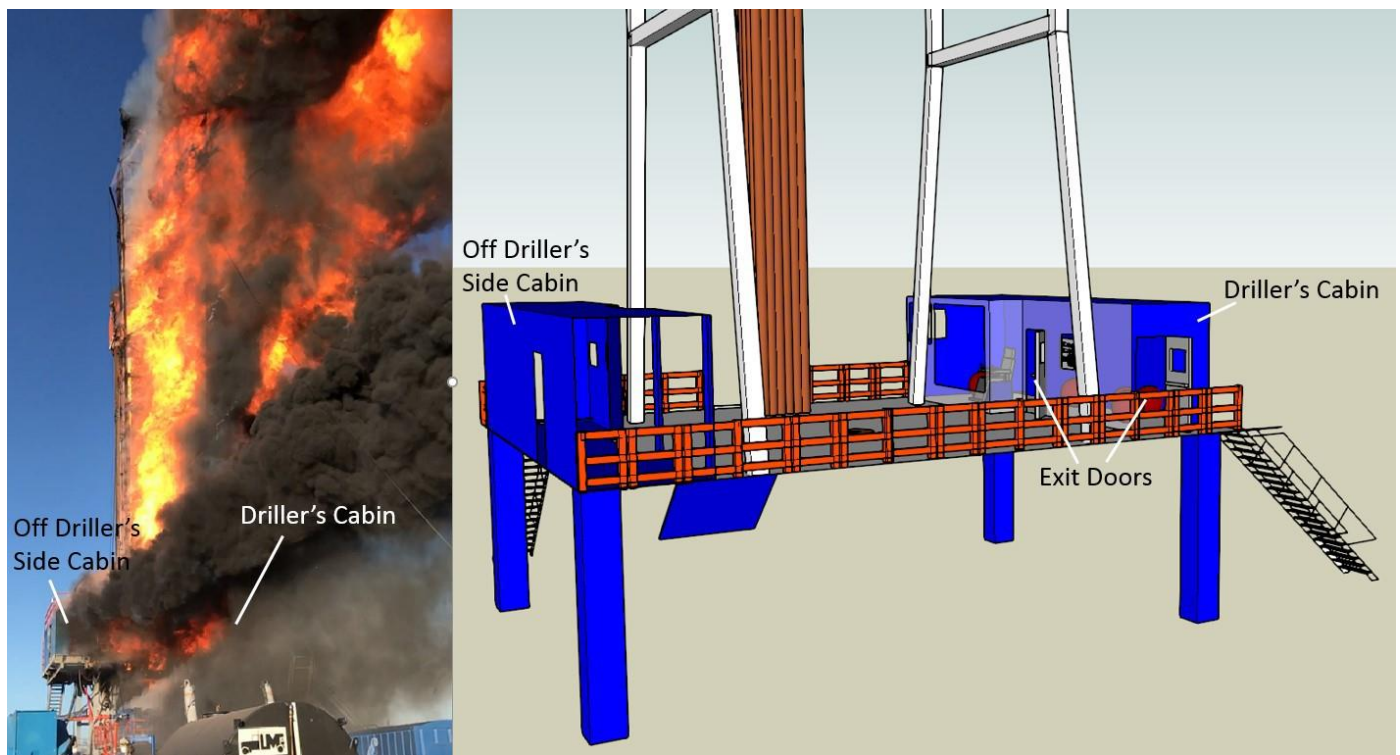
Figure 44. Both exits from the driller's cabin were engulfed by fire.
