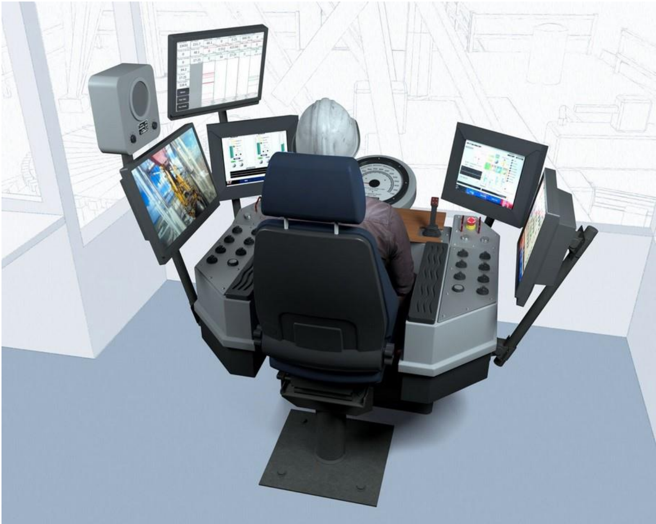
Figure 37. Depiction of driller console on Rig 219. The upper screen to the left of the driller displayed the aggregate of the drilling data.
