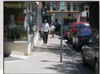
On-street parking creates a buffer between motor vehicle lanes and the pedestrian realm.
