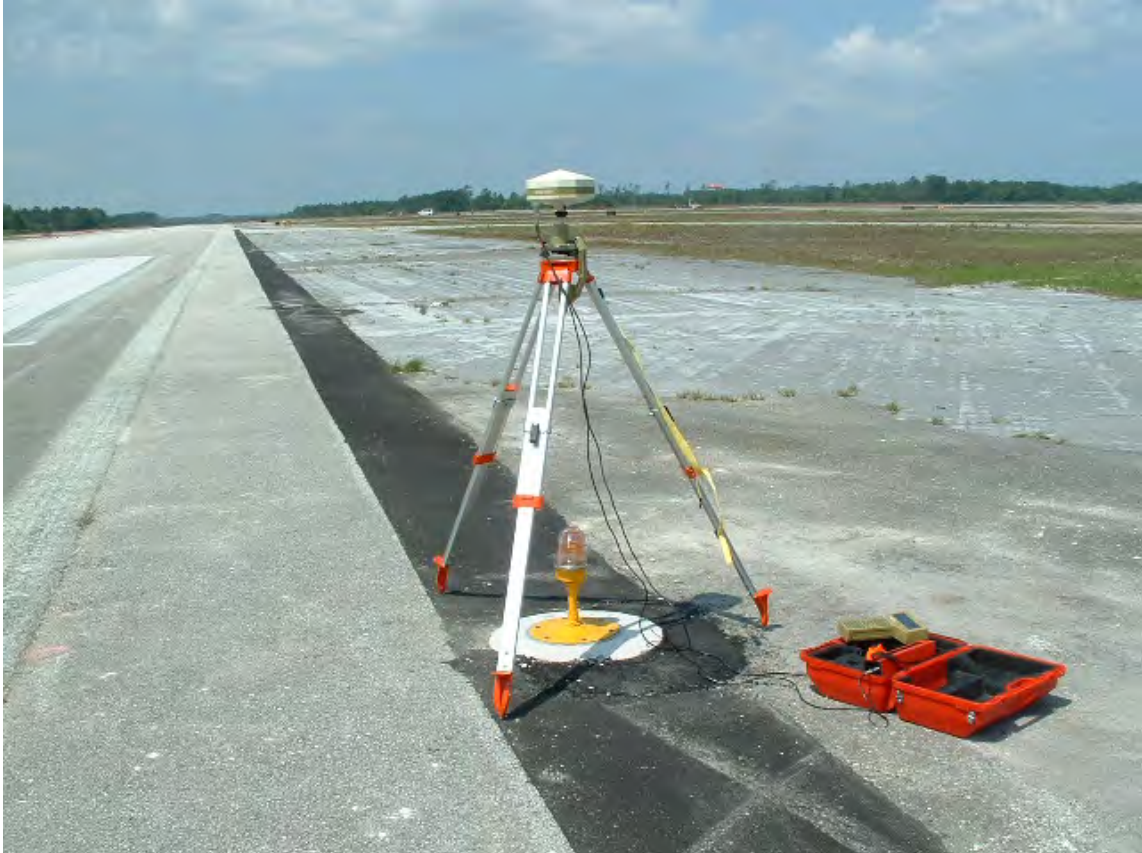
Figure 2-3. Airfield NAVAID positioning using Fast-Static GPS methods
