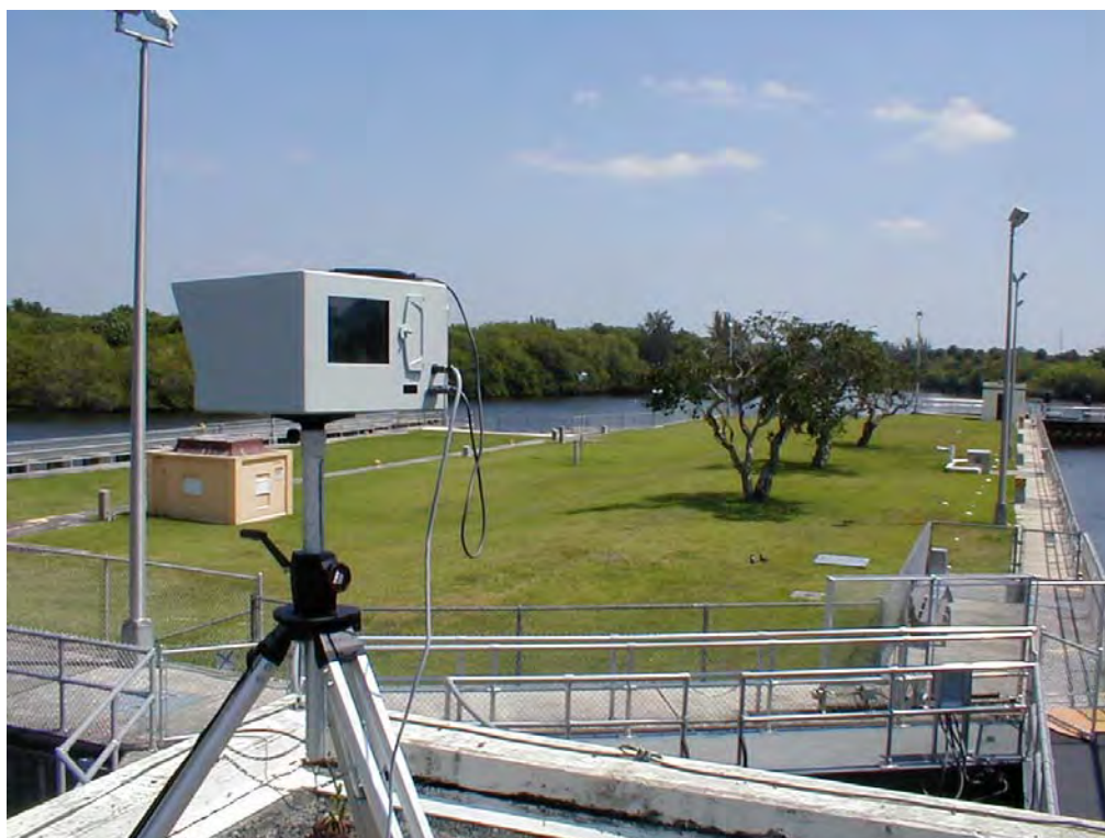
Figure 10-1. Optech ILRIS 3D laser scanner--detailed mapping of structures and facilities at St. Lucie Lock and Dam, Jacksonville District (Arc Surveying & Mapping, Inc.)
