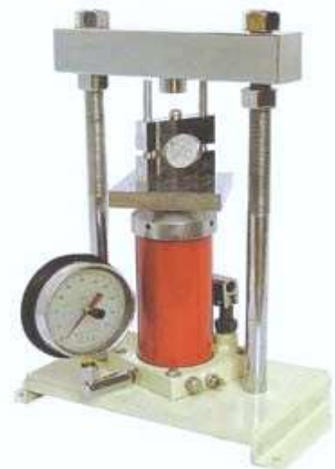
Figure 4.19. Brazilian test apparatus
