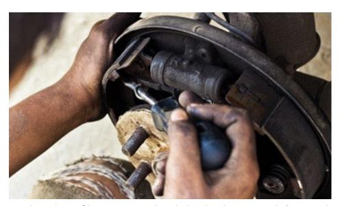
Asbestos is used as a loose fibrous mixture, bonded with other materials (e.g. Portland cement, plastics and resins) or woven as a textile. The range of applications in which asbestos has been used includes roofing, thermal and electrical insulation, cement pipe and sheets, flooring, gaskets, friction materials (e.g. brake pads and shoes), coating and caulking compounds, plastics, textiles, paper, mastics, thread, fibre jointing and millboard (1).
