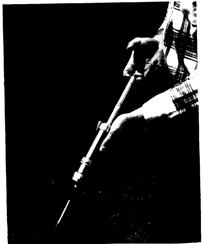
Photos 10a and 10b. Bendex-Gas Tec. H 2 S pump-style detectors. Photos by Ed Hickey.
