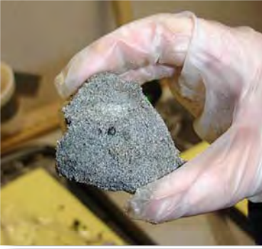
Sample of methane hydrate-saturated sandstone taken from Mt. Elbert Well in Milne Point Unit of Alaskan North Slope. (Courtesy of Mt. Elbert Science Team)
