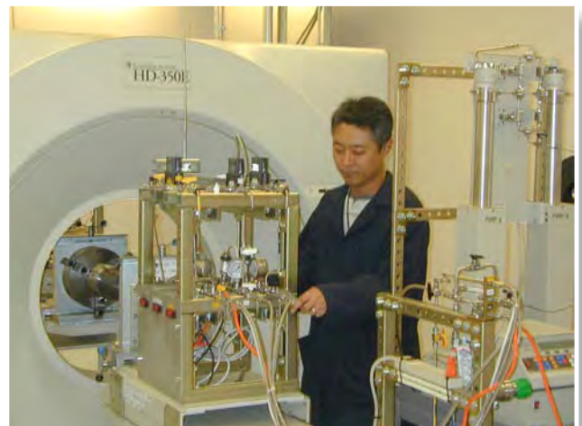
NETL researcher operates the X-ray CT scanner to observe methane hydrate formation in sandy sediments. (Courtesy of Yongkoo Seol, NETL)
