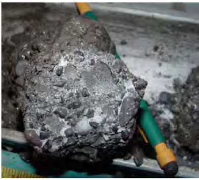
Methane hydrate-saturated coarse-grained sediment taken from core on Alaskan North Slope. (Courtesy of Timothy S. Collett, USGS)
