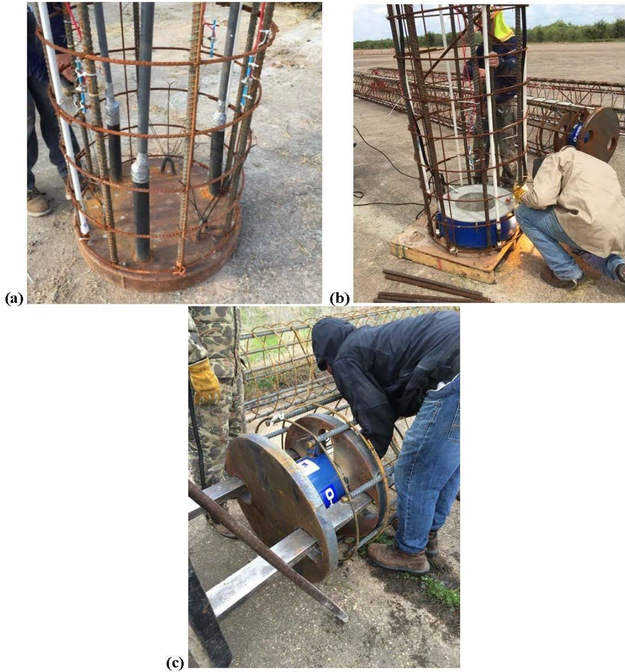
Figure 10.3: Bi-directional loading devices: (a) flat jack, (b) RIM Cell, and (c) O-Cell.
