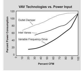
On existing VAV systems, convert airflow control from inlet vanes or outlet dampers to variable frequency drives (VFDs). Notice on the graph above how energy consumption using VFDs is far lower than using outlet dampers or inlet vanes.
