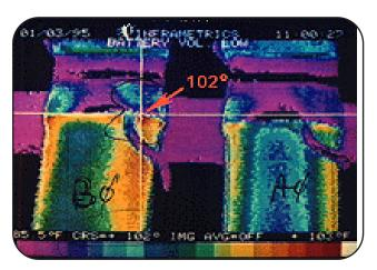
The hot spot on this infrared scan shows a problem with a control wire connection in a large generator breaker.
