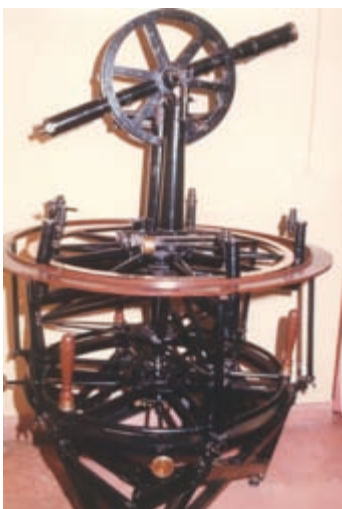
The 36 inch theodolite used on the Indian triangulation.
