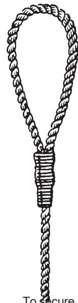
To secure splice – use whipping.
