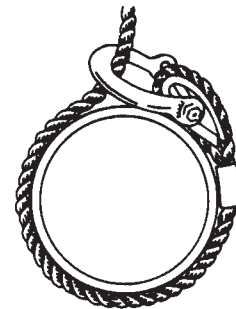
Correct – Shackle pin cannot turn.
