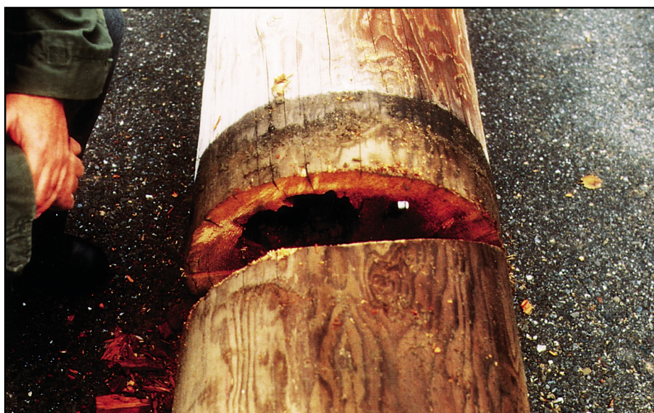
Figure 14-1 Pile that appears acceptable from the outside but that is decayed in the center.
