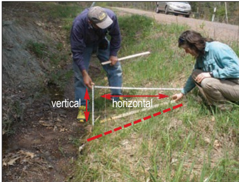
Figure 42: Ditch front slope example
