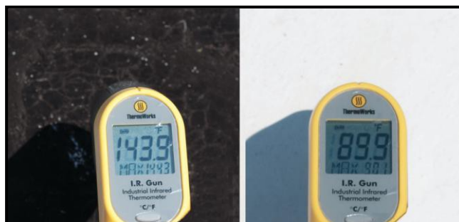
Figure 1: Dark vs. Cool Roof Surface Temperatures
