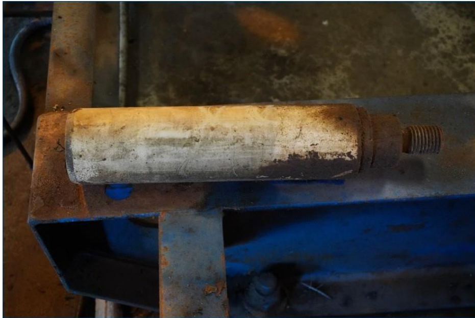
Figure 8. A spare ceramic plunger. (Credit: CSB)
