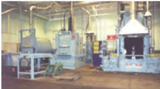
A quench furnace line for heat treating.
