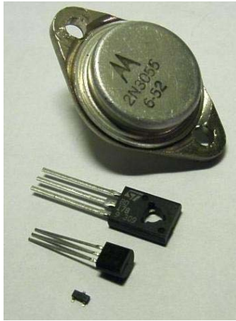
Figure 1b. Assorted discrete transistors. Packages in order from top to bottom: TO-3, TO-126, TO-92, SOT-23
