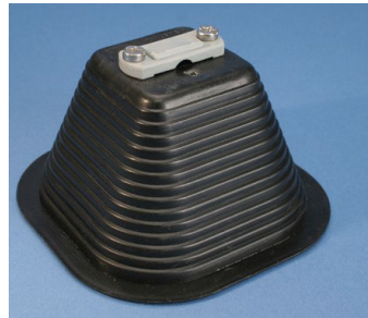
Figure 17. Stand-off bases are used to distance aluminum conductors from incompatible surfaces.
