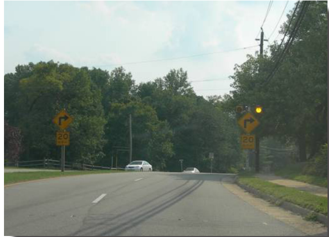
Typical arrangement of signs and flashing beacons.
