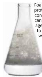
Foam in an oil system can lead to poor component protection and mechanical damage. Oil viscosity, contaminants, changes in surface tension and additives can all act as catalysts to the formation of foam. Anti-foam agents can stop foaming but require effective formulation to avoid **entrainment**—the entrapment of tiny bubbles within a fluid.
