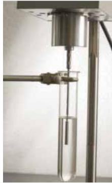
**Figure 3.3** Viscometer device used to determine a liquid's absolute or kinematic viscosity
