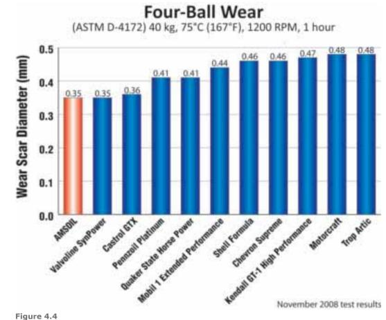
AMSOIL 10W-30 Synthetic Motor Oil demonstrates exceptional wear protection in the Four-Ball Wear Test.
