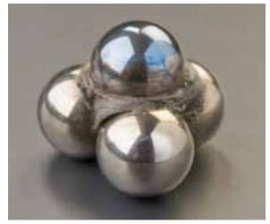
Figure 4.3 Example of welded test balls
