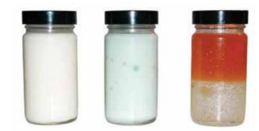
Figure 4.7 AMSOIL Synthetic Compressor Oil (shown far right), separates from water rapidly to inhibit rust formation and preserve wear protection.
