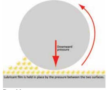
Figure 1.1 Hydrodynamic lubrication
