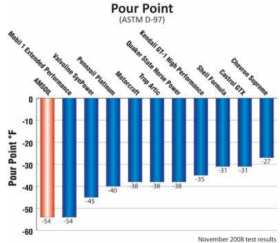
Figure 3.6 AMSOIL 10W-30 Synthetic Motor Oil exhibits an exceptionally low pour point (-54°F/-47.7°C) compared to most competitors.
