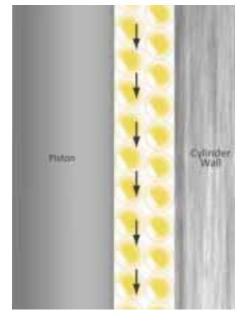
**Figure 3.7** Shear results when one layer of fluid moves in a direction different from another layer of that same fluid.
