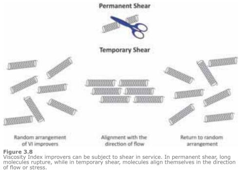
Mechanical activity within an engine creates shearing forces that can negatively affect a lubricant's protective viscosity. Even lubricants that provide consistent viscosity through a wide temperature range (a high viscosity index) are susceptible to shearing forces that reduce viscosity and load-carrying ability. Engines operating at high RPM and those that share a common oil sump with the transmission, like many motorcycles, experience high shear rates.
