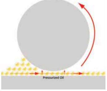
Figure 1.3 Hydrostatic-film lubrication
