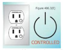
**Exception:** The marking is not required for receptacles controlled by a wall switch that provide the required room lighting outlets as permitted by 210.70.
