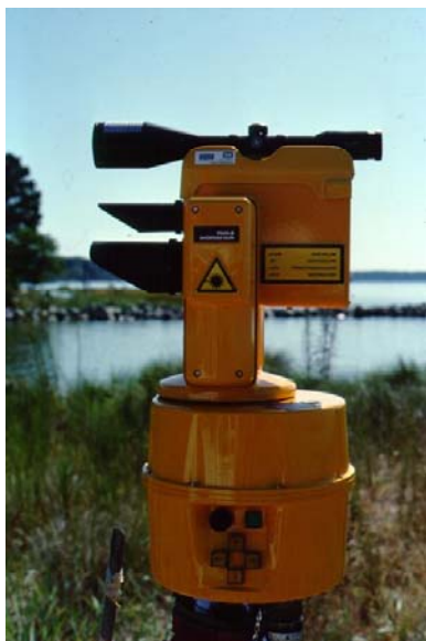
Figure 7-13. Various Range-Azimuth positioning instruments used in Corps (Norfolk District)
