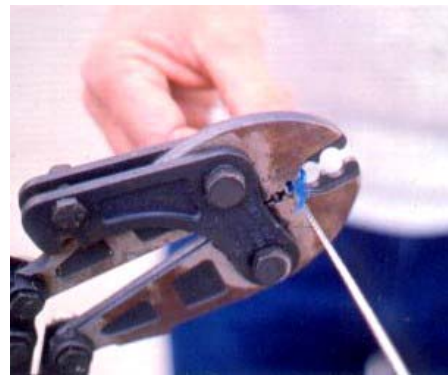
Figure 7-11. Tag line marking and calibration
