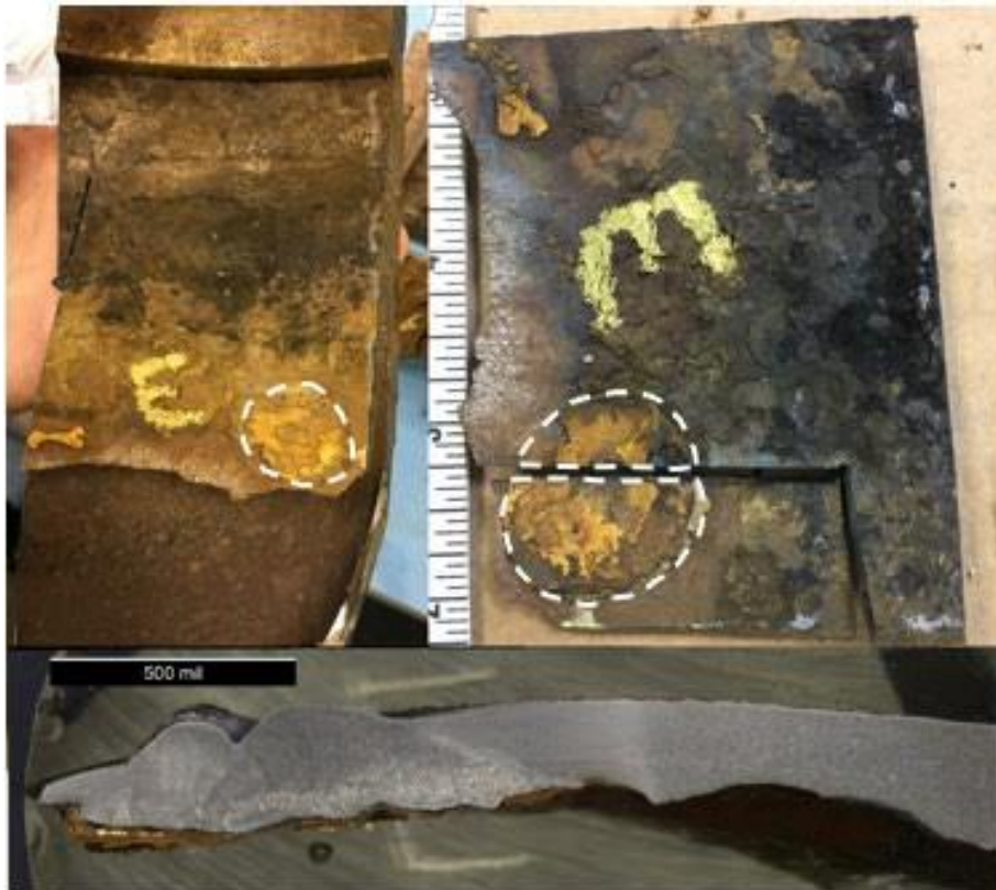
Figure 22. Plug weld found in the ring of steel still attached to the shell, cross-sectioned. (Credit: CSB)
