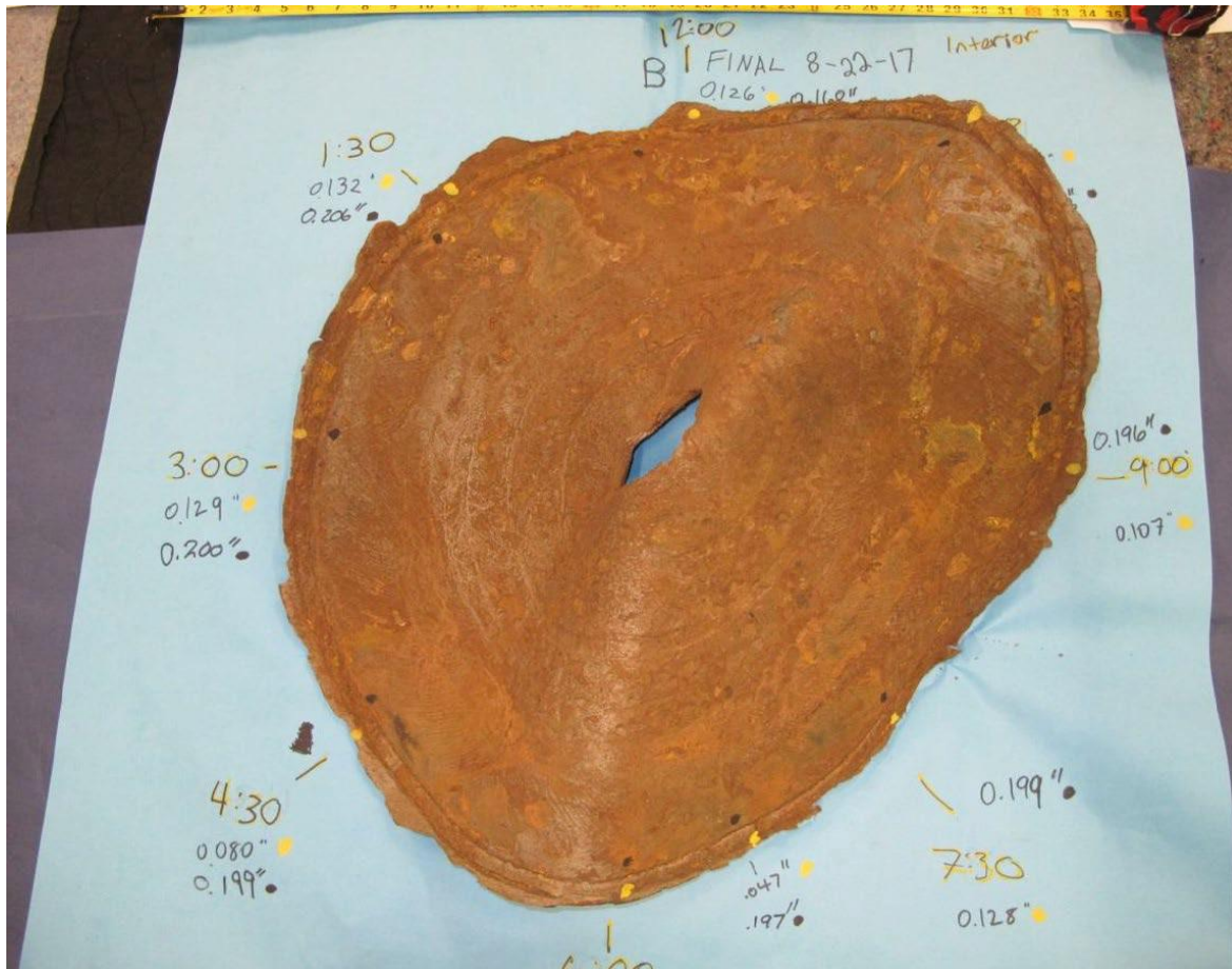
Figure 19. Thickness comparison on either side of patch-to-ring weld. (Credit: CSB)
