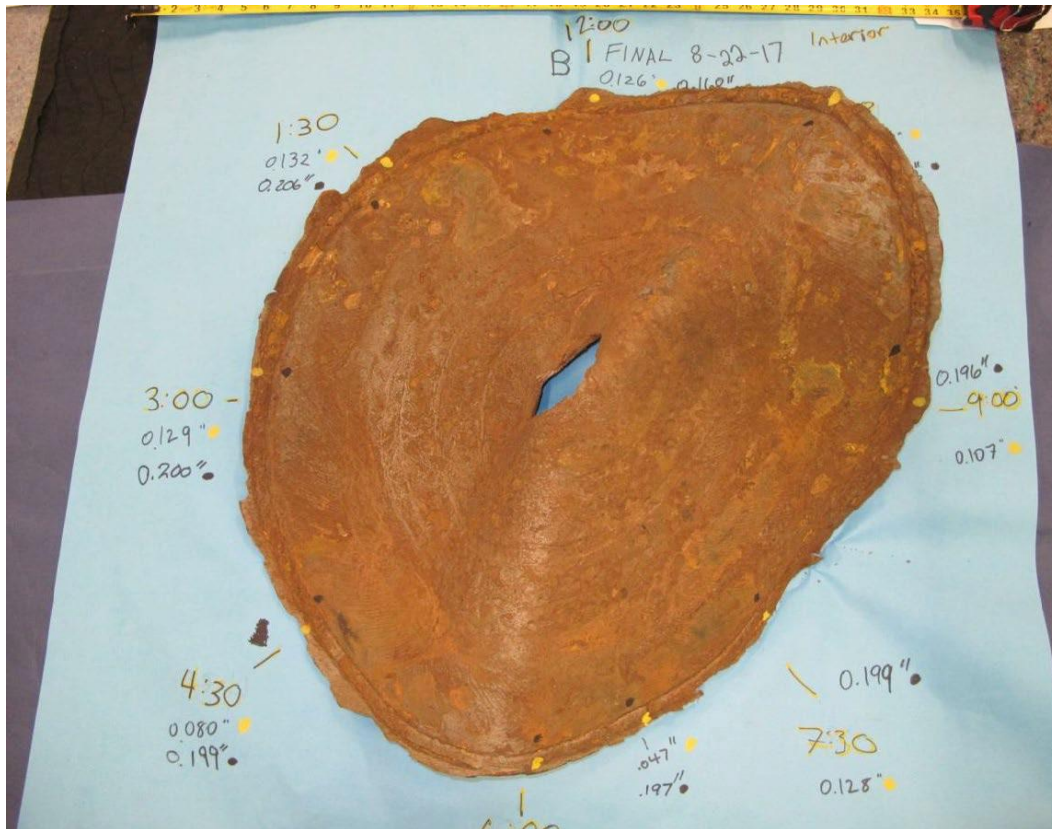
Figure 34. Thickness comparison on either side of patch-to-ring weld. (Credit: CSB).
