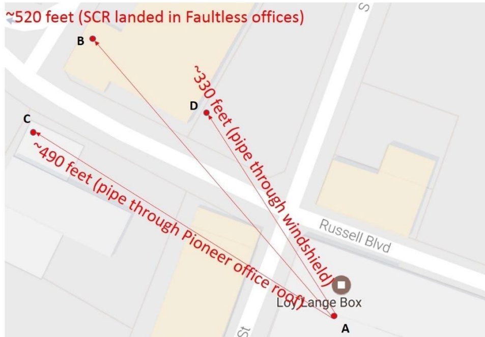
Figure 12. Debris map from incident. (Credit: Google, annotations by CSB)
