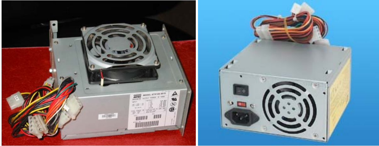
(a) Enclosed Frame Internal Power Supplies
