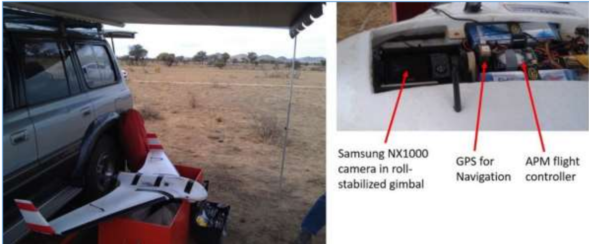
Figure 4. X8 fixed wing image acquisition platform
