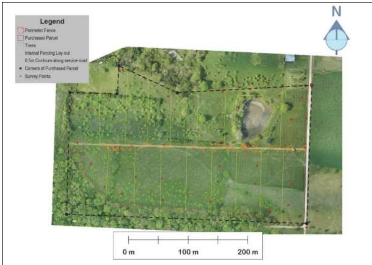
Figure 20. Vector data superimposed on orthophoto with GSD of 12.5 mm
