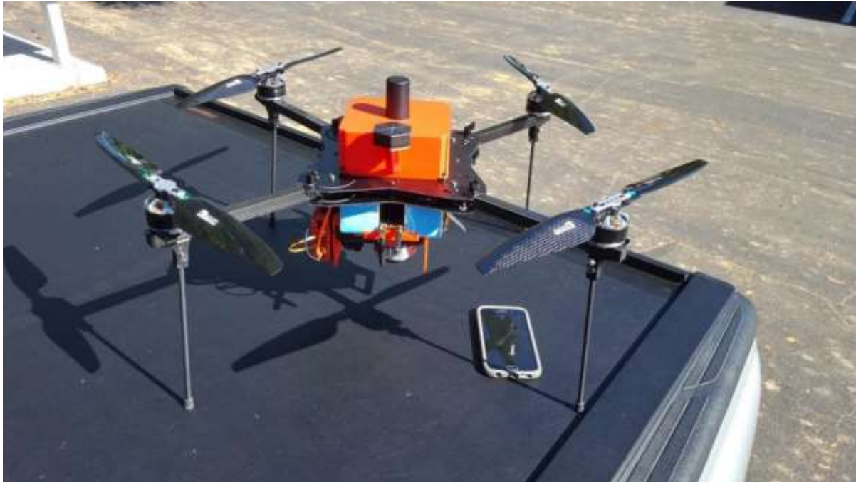
Figure 13. Survey quad copter equipped with a dual frequency V-Map GNSS receiver for accurate determination of CEPs
