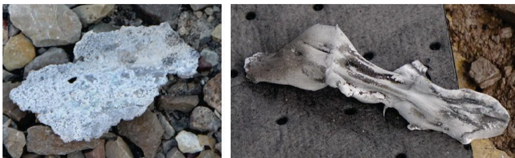
Figure 21. Aluminum Parts. The picture on the left shows an aluminum part from the MP odorizer involved in the May 24, 2017, incident that appears to have general corrosion. The photo on the right shows an aluminum part from the MP odorizer involved in the June 20, 2017, incident that appears to show signs of melting from heat. (Credit: MRR (left), SPSI (right)).
